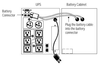
Figure 15. External Battery Connections (120V Model Shown)
